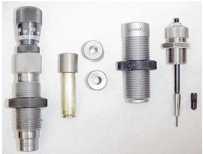
Superior Shooting Systems Inc. custom 6mmXC die set components [left to right] Redding competition bullet seater / gauging bushing in use on case / .265 and .267 neck/shoulder sizing bushings / sizing die body / decapping stem with tapered expander installed, bushing retainer / decapping pin retainer to replace expander after initial sizing
