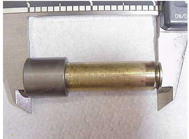
Fired case in the caliper with the gauging bushing in place.
